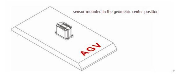
2. The installation of the instrument should be kept parallel to the surface of the measured object, and reduce the influence of the dynamic and acceleration on the angle meter. Incorrect installation will lead to measurement errors, with particular attention to "surface" and" line "
