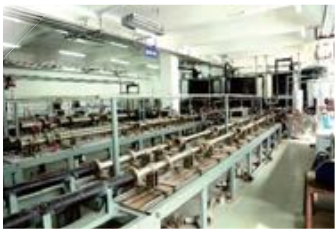
Calibration for Ultrasonic Flowmeter
