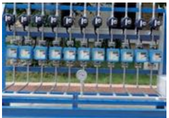
Rotameter system for mixed gas measurement
