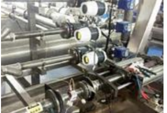
Magnetic flowmeter in calibration
