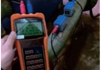
Ultrasonic flow meter for clean water measurement
