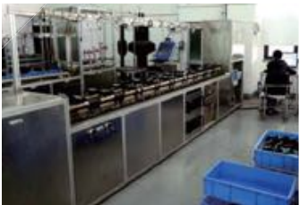
Calibration for Ultrasonic Heat Meter
